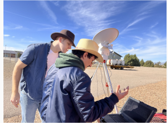
EMU APEX at the ground station setting up the tracking satellite antenna for downloading data about 40 miles to the east of the launch site. View is toward the balloon with the dish pointing at the weather balloon. From left: Miles Mercier, Axel Cartin-Paez.
